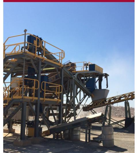
**Crushed Ore Sampling System**
